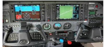
\*All of these aircraft are equipped with the Garmin G-1000 advanced computerized instrument panels with GPS moving map navigation.
